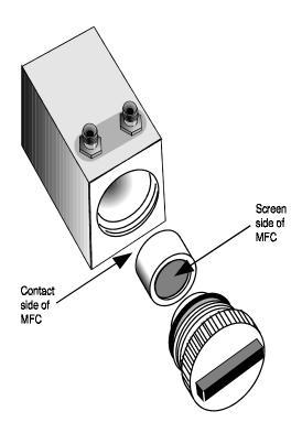
Figure 5-2: Exploded View of MFC and Cell Block
